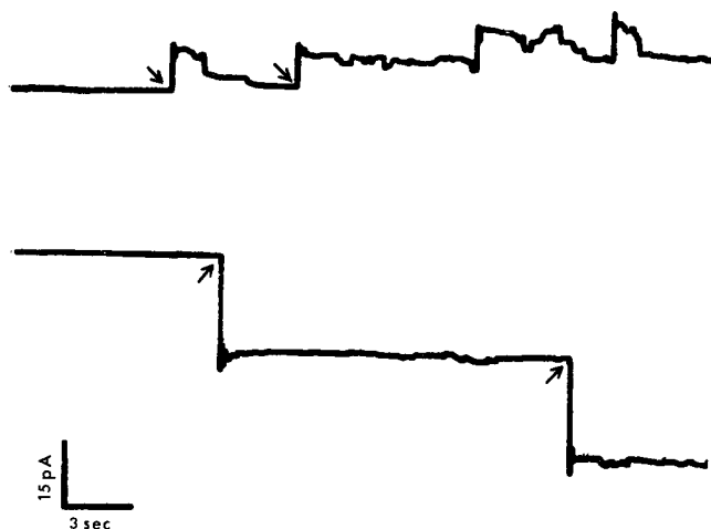
Fig. 1. Current steps arising when small amounts of hemocyanin are added to a bilayer. Hemocyanin concentration, 2 \cdot 10^{-8} g/ml. Upper trace was obtained at +100 mV, lower trace was obtained at -100 mV. In the upper trace, formation steps of approx. 9 pA are seen, followed by small on-off steps. The lower trace shows two larger formation steps of approx. 20 pA. Membranes were formed in 100 mM KCl, pH 7. Temperature, 26 °C.
